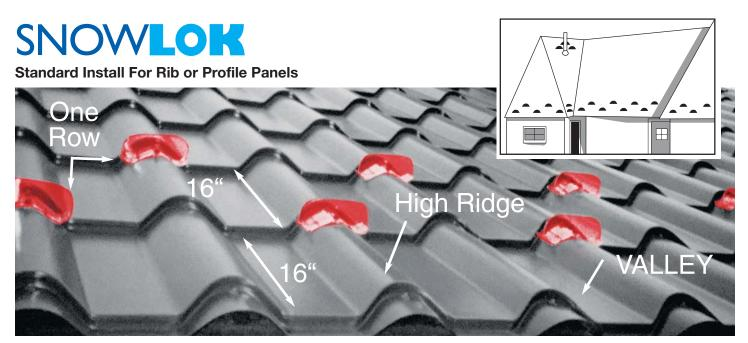
First row should start 16" from the eave (not the over hang), alternating up and down on each rib in a staggered pattern.
