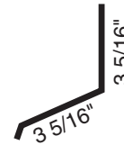
Wall Flashing No Return
